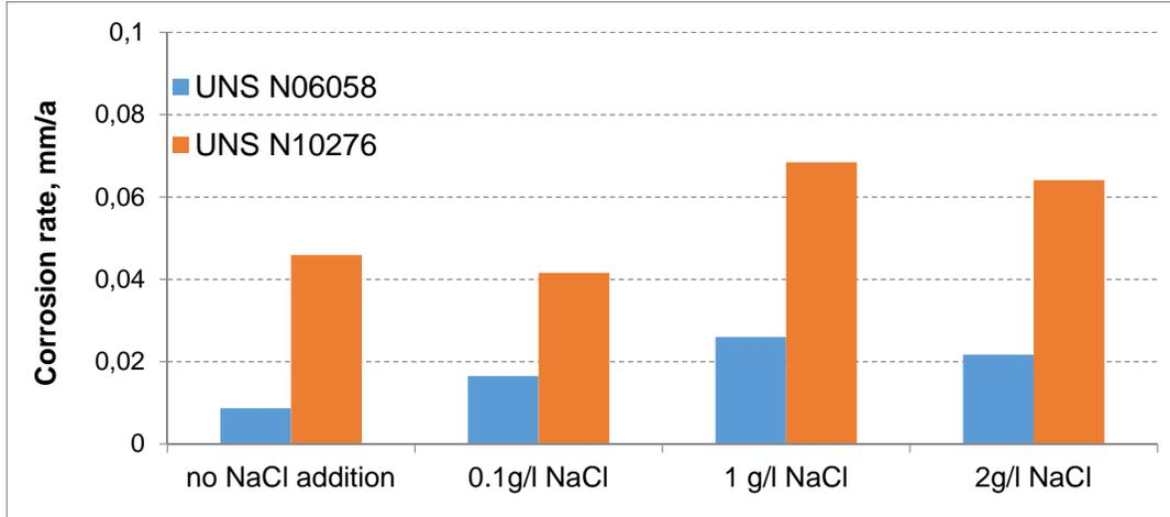
**Fig. 8:** Corrosion rate (mm/a) of alloy UNS N06058 test samples in 50 % acetic acid + 40 % formic acid + 5 % sulphuric acid at 95 °C without and with different additions of chlorides in form of NaCl in comparison to alloy UNS N10276. Testing period for immersion 24 hrs.
