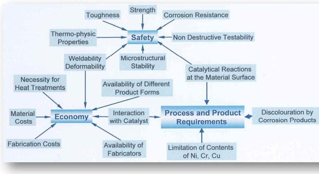
**Fig. 1:** Criteria for material selection in the process industry (from J. Korkhaus, *ACHEMA* 2006 [1]).
