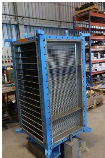
**Fig. 9:** Application of alloy UNS N06058 as material of construction for: (left side) heat recovery systems for indirect heat transfer in a FGD plant and (right side) plate heat exchangers for hydrochloric acid in a chemical plant (equipment manufactured by ZIEMEX).
