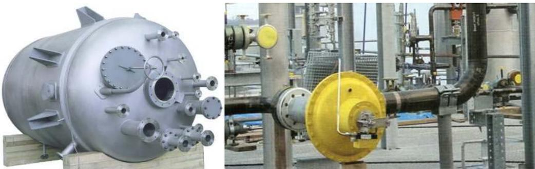
**Fig. 6:** Application of alloy UNS N06059 as material of construction for: (left side) reactor for the production of catalysts and (right side) piping for a HP-technology melamine plant.
