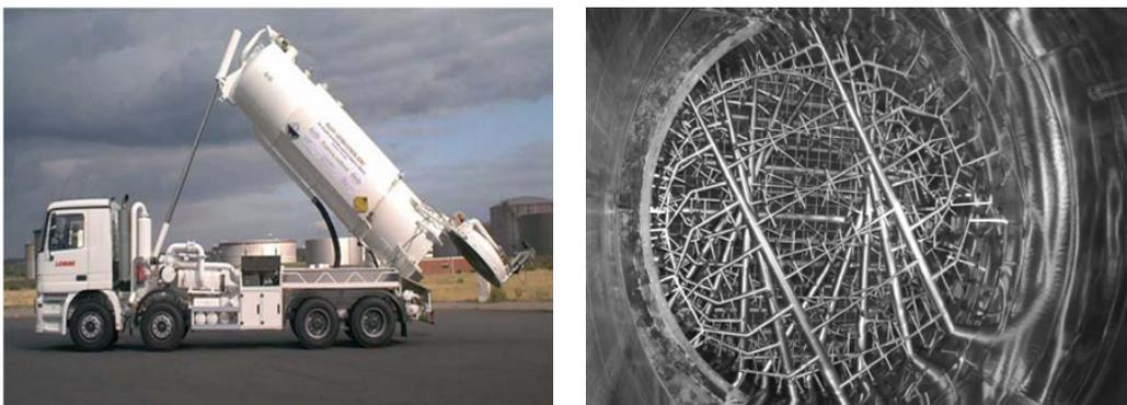
**Fig. 10:** Application of alloy UNS N08031 as material of construction for: (left side) road truck for the transport of waste acids and solvents, mainly waste sulphuric acid (Lobbe, Germany) and (right side) quencher spray system after 10 years in service in a flue gas scrubber.
