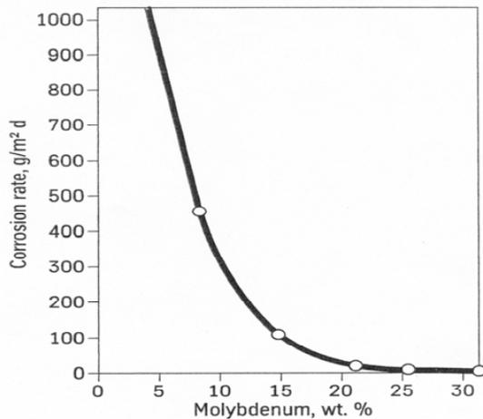
**Fig. 4:** Corrosion rate of binary nickel-molybdenum alloys in boiling 10 % hydrochloric acid as function of the molybdenum content (from K. E. Volk, 1970 [7])
