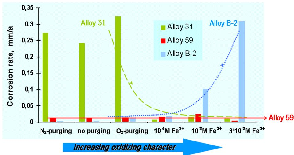
**Fig. 13:** Corrosion behaviour of a nickel-chromium-molybdenum alloy (alloy 59), a nickel-chromium-iron-molybdenum-copper alloy (alloy 31) and a nickel-molybdenum alloy (alloy B-2) in an aqueous solution with increasing oxidizing character
