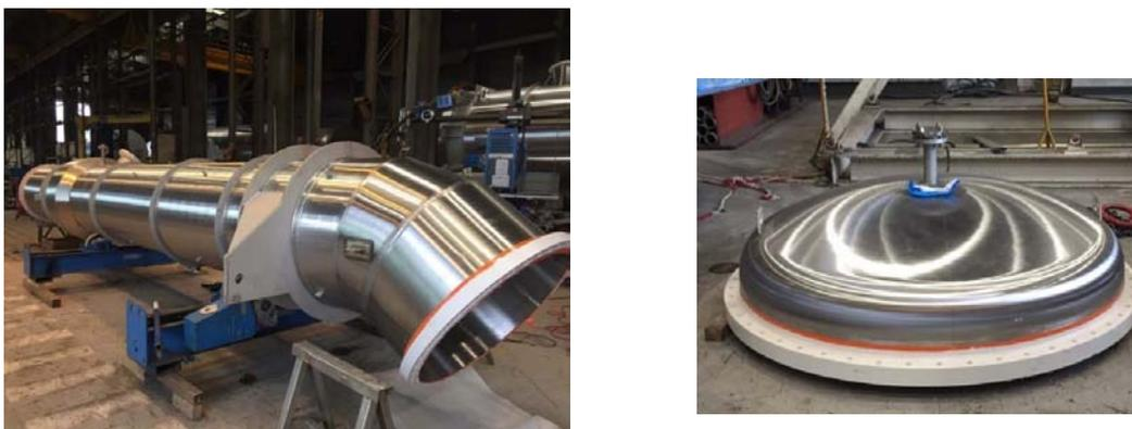
**Figure 12:** Example of application of alloy UNS N08034 for evaporators in the salt industry. Equipment manufactured by ZIEMEX.
