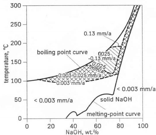
**Fig. 2:** Corrosion resistance of unalloyed nickel (UNS N02200) in sodium hydroxide as a function of concentration and temperature (from W. Z. Friend, 1980 [6])
